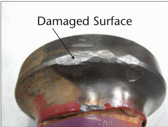
FIGURE 5 - Damaged flange backside
