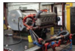
All repaired pumps are tested to full power before returning to the customer.
