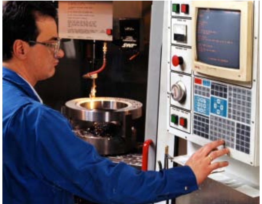
Top: CNC machining of a part from a CMM generated drawing
