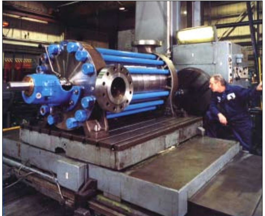
Top right: Final alignment checks on multistage pump
