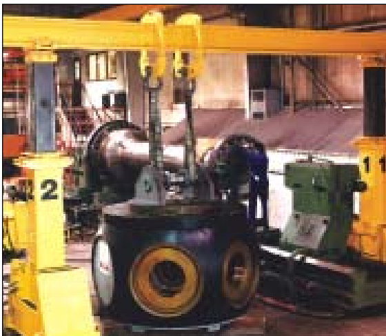
Below: Our 125-ton capacity portable Lift-n-Lock gantry crane maneuvers a 36-ton hub for a Kaplan Hydro turbine
