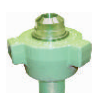
Fig. 2202 Green Nut - Green Subs Especially for sour gas service; with heat-treated components, fluoroelastomer seal rings. For service to 15,000 psi NSCWP*.
