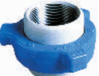
Fig. 206 Blue Nut - Gray Sub A precision metal-to-metal seal plus O-ring seal for air, water, gas, oil and mud service to 2,000 psi NSCWP*.
