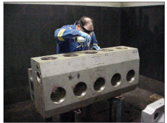
Fluid ends are thoroughly inspected by trained technicians to determine the scope of work required to repair the cylinder.
